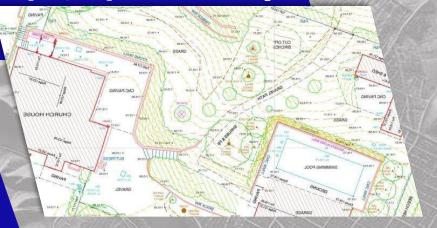
A topographical survey, often called a topo survey, is a detailed analysis of the natural and artificial features of a specific area of land. These surveys are crucial for projects involving construction planning, infrastructure development, environmental assessments, and urban planning. By mapping and observing spot heights thus contours and elevation, and surface features, topographical surveys provide essential data for various engineering and architectural projects.
